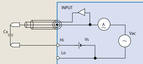
Contact Failure Detection Circuit
