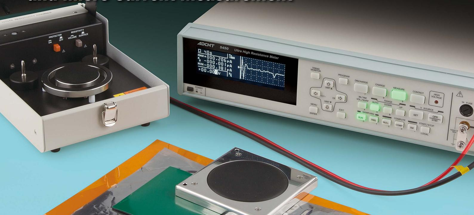
The 5450/5451 is a state-of-the-art ultra high resistance meter with 5½-digit display that integrates ADC's traditional technologies and new DC amplifier technologies. It was designed for ease of use so that anybody who operates this instrument can get the same measurement results. The 5450/5451 will be the new standard for insulation resistance measurement or micro current measurement of various kinds of insulating materials or semiconductors.
